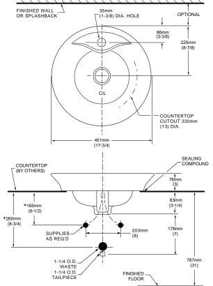
NOTES: \*DIMENSIONS SHOWN FOR LOCATION OF SUPPLIES AND "P" TRAP ARE SUGGESTED. FITTINGS NOT INCLUDED WITH FIXTURE AND MUST BE ORDERED SEPARATELY. FOR COUNTERTOP CUTOUT AND INSTALLATION INSTRUCTIONS USE TEMPLATE SUPPLIED WITH SINK.
